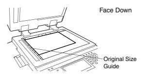
• Place a book or an original Face Down on the Platen Glass, aligning it with the arrow mark on the original size guides.
